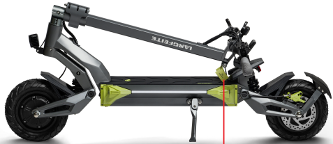
Stem and deck can be fixed with the lock
