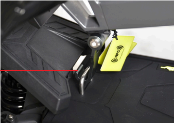
Stem and deck can be fixed with the lock
